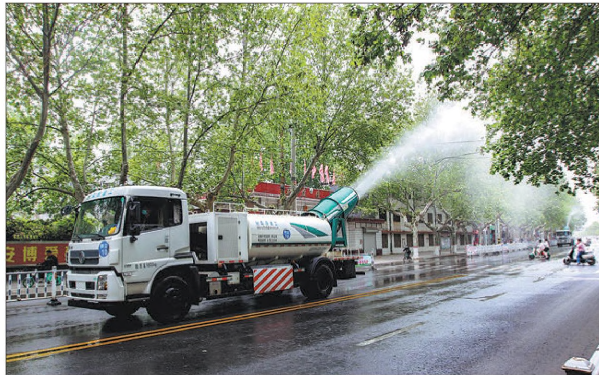
A vehicle equipped with water cannon is seen in Jiaozuo, Henan province, on April 11. The water cannon can disperse water into the air to control dust and reduce air pollution. CHENG QUAN / FOR CHINA DAILY
