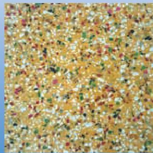
A tile made of waste ceramics in Jingdezhen. PROVIDED TO CHINA DAILY
