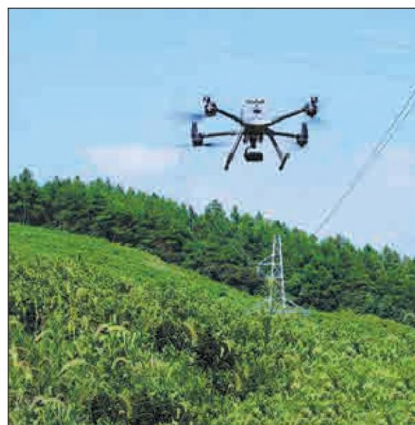
Below: United Aircraft's drone Q20 is used to inspect grid systems in Wuhu, Anhui province. PHOTOS PROVIDED TO CHINA DAILY
