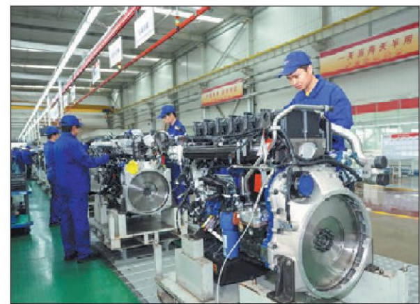
Workers assemble gas-driven engines at Weichai Group in Weifang, Shandong province, in March. PROVIDED TO CHINA DAILY
