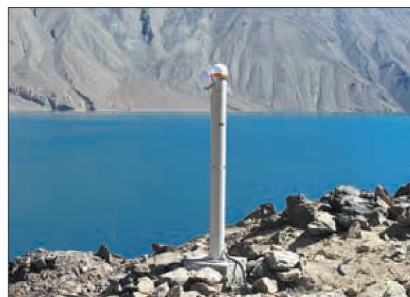
From left: Members of the Chinese-Tajik scientific team climb to the Lake Sarez area in 2021. A monitoring tower on the bank of the lake collects data on deformations on the dam.
