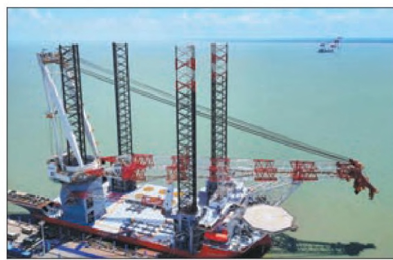
Wind Peak, an offshore wind turbine installation vessel, docks at a shipyard in Qidong, Jiangsu province, on Thursday. The vessel is able to transport and install seven complete 15 megawatt turbine sets per load. XU CONGJUN / FOR CHINA DAILY
