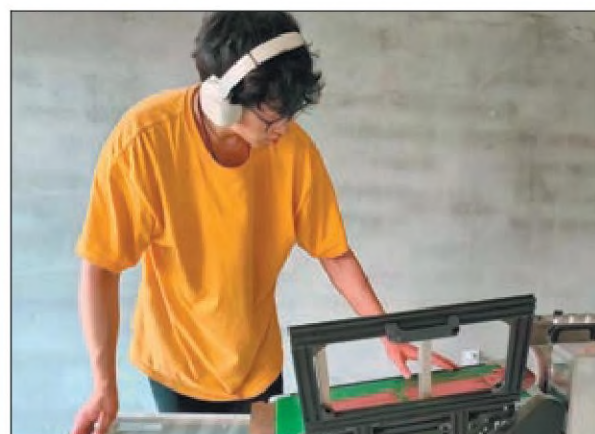
Left: Zhang Junfeng uses a cutting machine to trim the extruded incense to standardized lengths, ensuring neat and even ends. Middle: Weng Jianzhi selects and prepares ingredients for incense at his workshop in Zhoushan, Zhejiang province. PHOTOS PROVIDED TO CHINA DAILY Right: A vendor displays a variety of incense in Hangzhou, Zhejiang province, in June. WENG XINYANG / XINHUA
