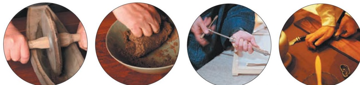
From left: All aromatic ingredients are ground into a fine powder to ensure even burning and a smooth texture. They are then rolled into a dough-like consistency. After drying the uneven ends are trimmed, and the sticks are smoothed. PHOTOS PROVIDED TO CHINA DAILY
