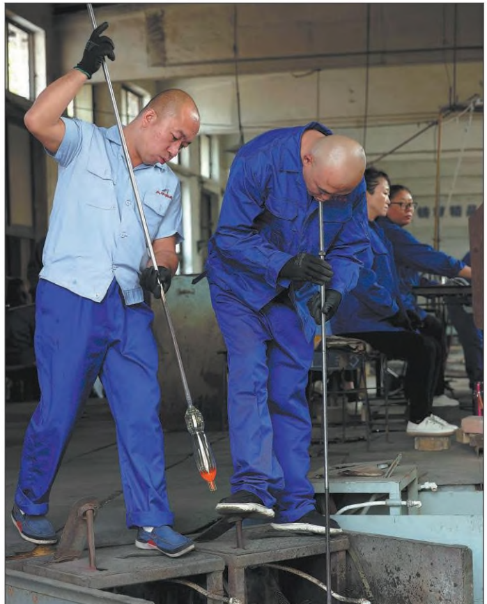
Left: Two glassworkers blow molten glass through blowpipes at the factory. Right: Workers tidy up handmade wineglasses in the factory.
