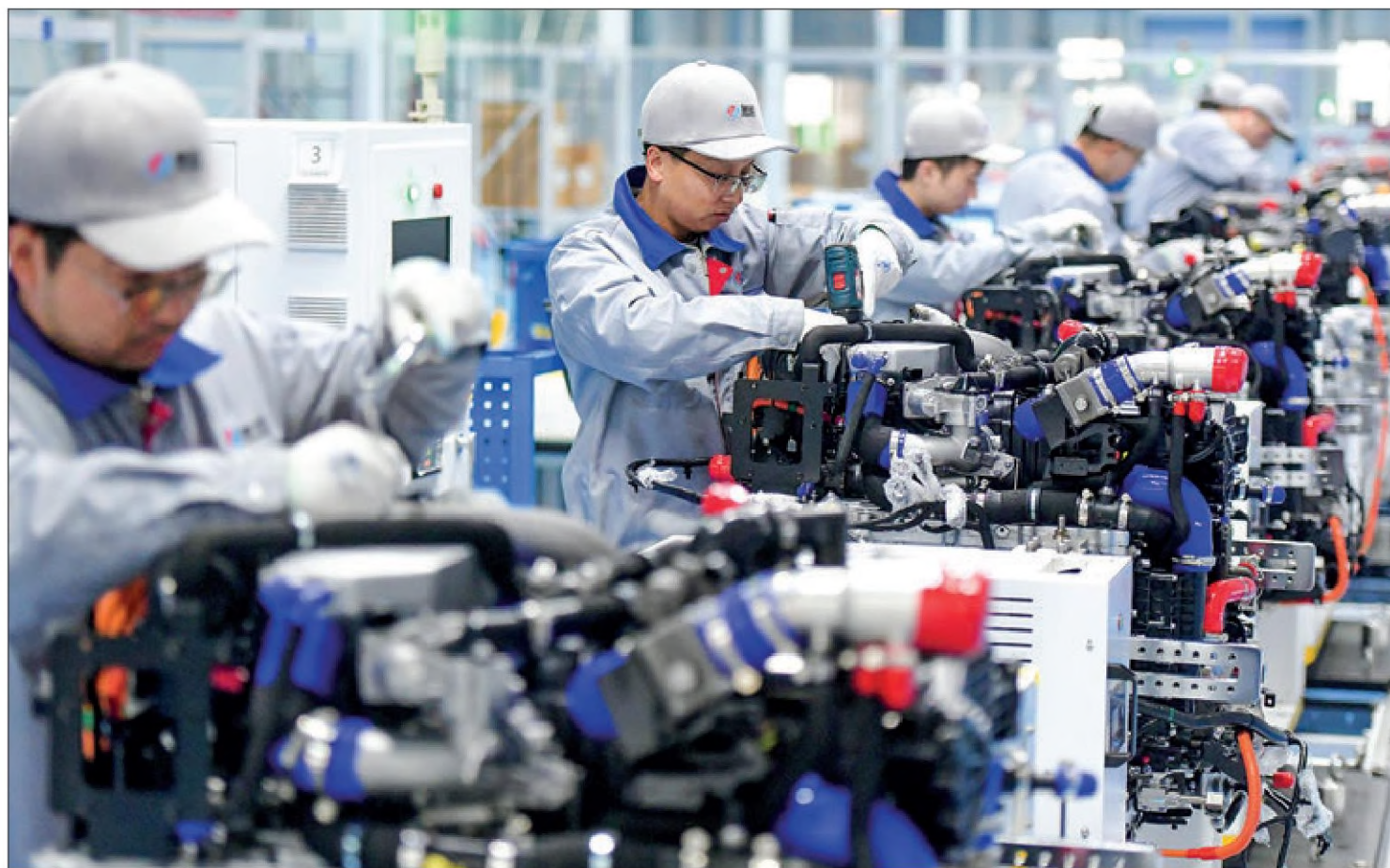
Workers assemble hydrogen fuel cell engines on a production line in Luoyang, Henan province in November. ZHANG YIXI / FOR CHINA DAILY
