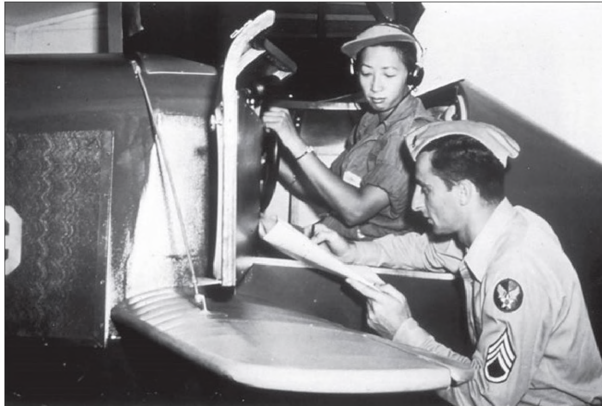
Hazel Ying Lee reviews her performance after a session on a Link trainer, a mechanical flight simulator used to train pilots in navigation and instrument flying. PHOTOS PROVIDED TO CHINA DAILY
