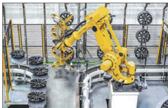
An automated production line at the CITIC Dicastal Morocco plant, Africa's first Lighthouse Factory. PROVIDED TO CHINA DAILY
