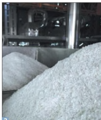
Recycled bottles usually undergo the following procedures before they become granulated plastics (Photo 5) and are made into clothes or bags by companies like HowBottle. Compacted plastic bottle blocks (Photo 1); Sorting by color (Photo 2); Shredding (Photo 3); Granulating (Photo 4). PHOTOS PROVIDED TO CHINA DAILY
