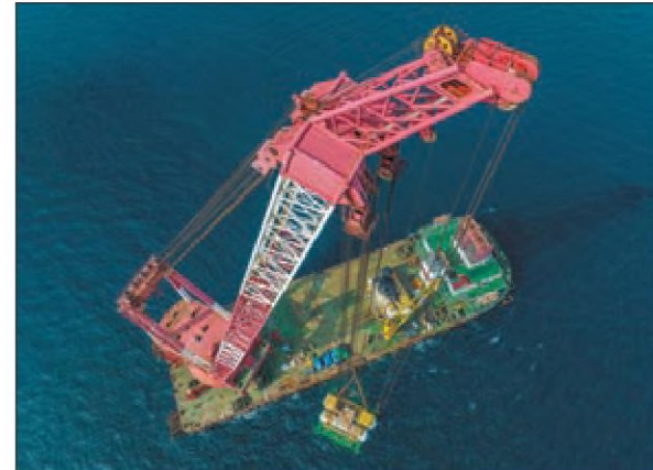
A new data module of the underwater intelligent computing cluster is deployed off the coast of Hainan on Feb 18. PROVIDED TO CHINA DAILY
