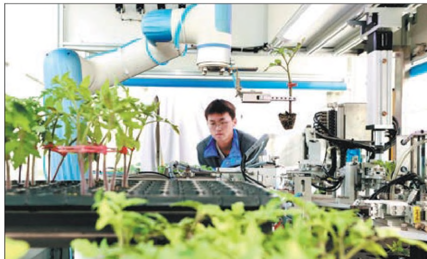
An automated robot grafts tomato seedlings in a digital seeding farm in Tongxiang, Zhejiang province, on Feb 19. The process only takes three seconds for each seedling, with a survival rate of 99 percent. WANG JIANLONG / ZHEJIANG DAILY
