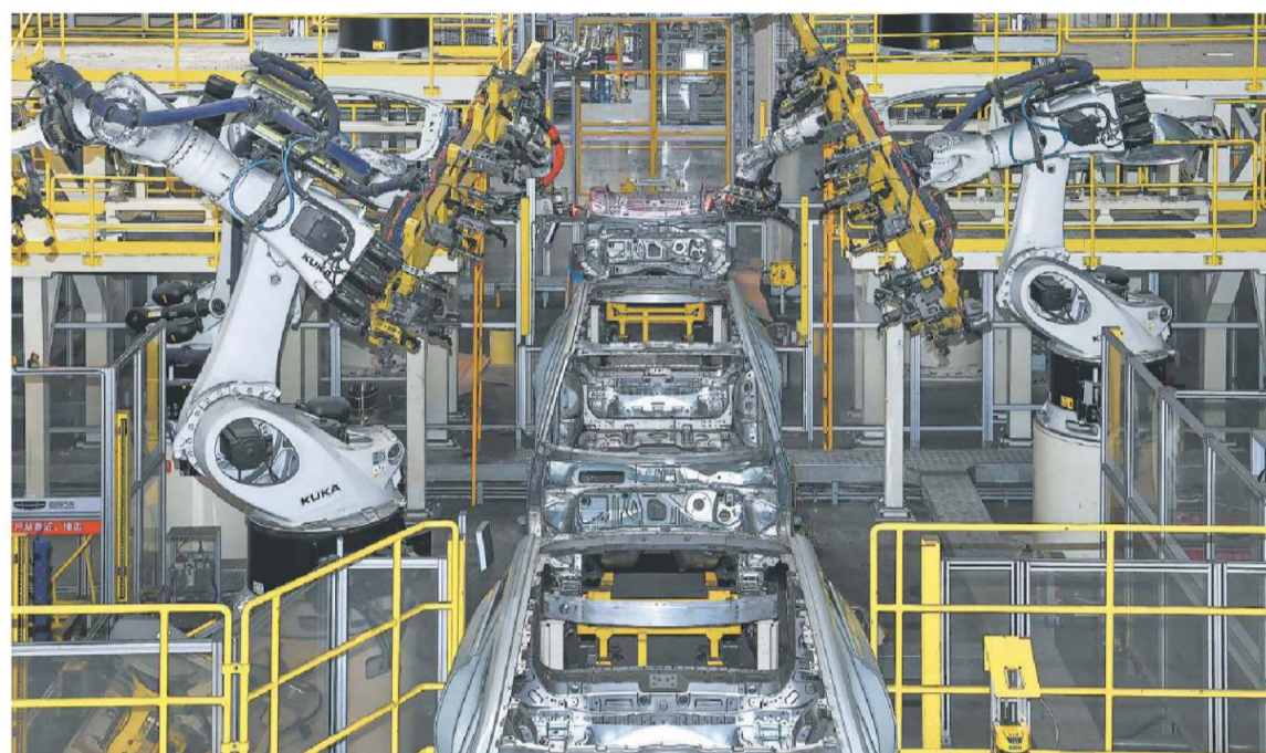
An automated welding line operates at an automobile plant in Baoji, Shaanxi province, on Feb 26. ZOU JINGYI / XINHUA
