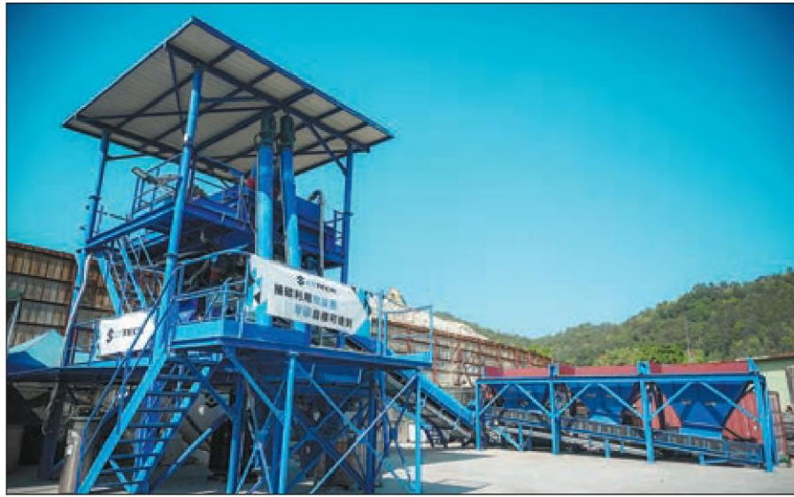
Left: At a pilot project, a cylinder of liquefied CO 2 is injected into cement to make concrete, which could reduce the use of high carbon-footprint cement. It was co-initiated by CS Tech Solution, a local cement factory and the Hong Kong Productivity Council. Right: A bench printed by a 3D concrete printer is seen featured with recycled tiles and planks. PHOTOS BY ANDY CHONG / CHINA DAILY
