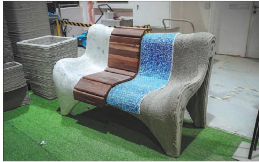
Left: At a pilot project, a cylinder of liquefied CO 2 is injected into cement to make concrete, which could reduce the use of high carbon-footprint cement. It was co-initiated by CS Tech Solution, a local cement factory and the Hong Kong Productivity Council. Right: A bench printed by a 3D concrete printer is seen featured with recycled tiles and planks. PHOTOS BY ANDY CHONG / CHINA DAILY
