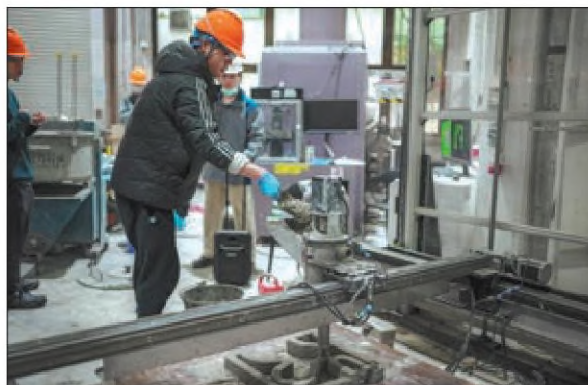
Left: A staff member at the PolyU-NAMI 3D Concrete Robotic Printing Research Centre operates a 3D concrete printer during a demonstration at PolyU. Middle: A compact CS Tech Solution's carbon-capturing system is ready for operation. Right: Poon Chi-sun, director of the Research Centre for Resources Engineering Towards Carbon Neutrality at Hong Kong PolyU, introduces a concrete-3D-printed art installation for Valentine's Day. Visitors to the department's atrium were allowed to take selfies in front of the object.
