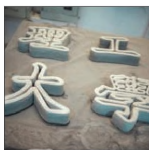
A 3D printer used concrete injected with CO 2 to produce the Chinese characters for Hong Kong's PolyU seen above. The CO 2 reacts with calcium to quickly harden the concrete, allowing it to be printed in varying shapes.
