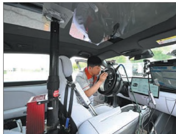
A technician installs a steering robot for an upcoming test of an intelligent connected vehicle in July in Tianjin. SUN FANYUE / XINHUA
