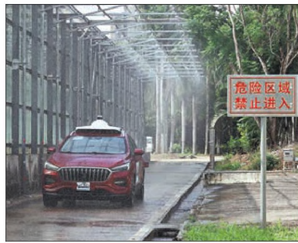
A car undergoes an automated driving test in simulated rainy conditions in Haikou, Hainan province, on May 8. GUO CHENG / XINHUA
