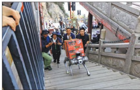
A robot dog carries supplies up stairs at Laojun Mountain scenic area in Luoyang, Henan province, on Wednesday. Equipped with advanced artificial intelligence algorithms and sensors, the robot can carry a load of up to 120 kilograms while at a standstill and a load of 40 to 60 kg while on the move. PROVIDED TO CHINA DAILY
