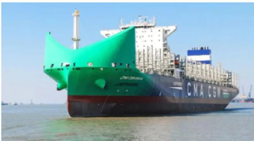
CMA CGM is adding a larger wind deflector to improve fuel efficient on its containerships (CSSC)
