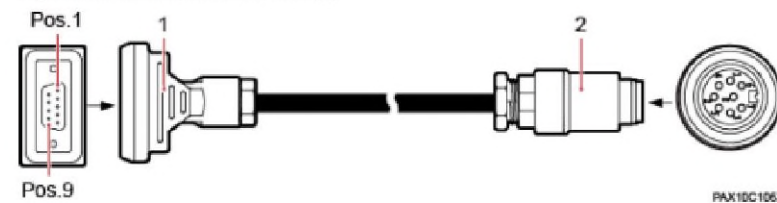
Figure 2 AISG multi-wire cable (2)
