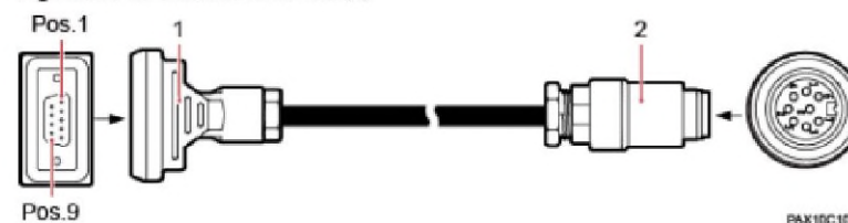
Figure 2 AISG multi-wire cable (2)
