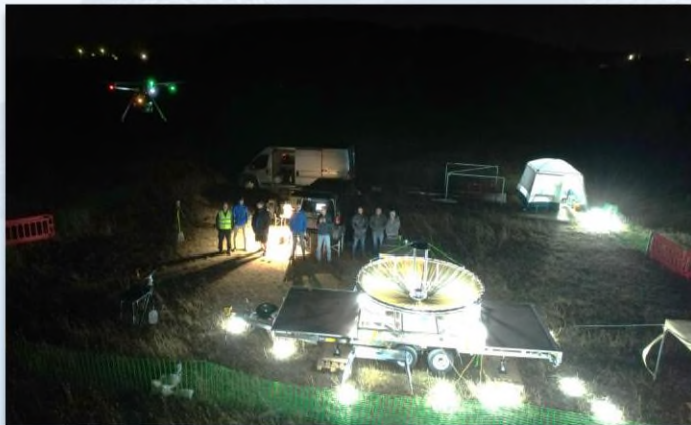
Oxford Space Systems – UK, Harwell Campus 3m and 5 m deployable – X band. Prototype validation and alignment of struts.
