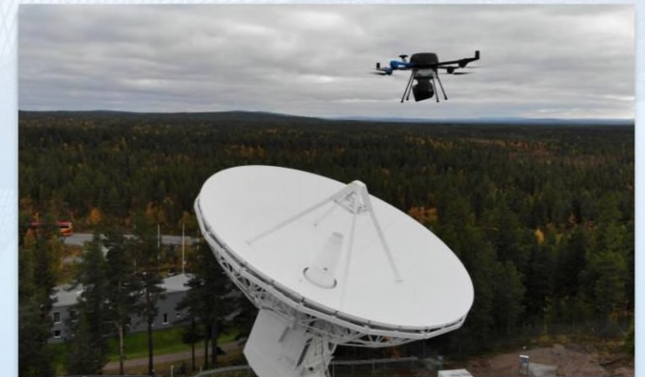
ESA ESOC – Sweden, Kiruna 15m earth station – X band. Tracking verification and SUM/DELTA measurements
