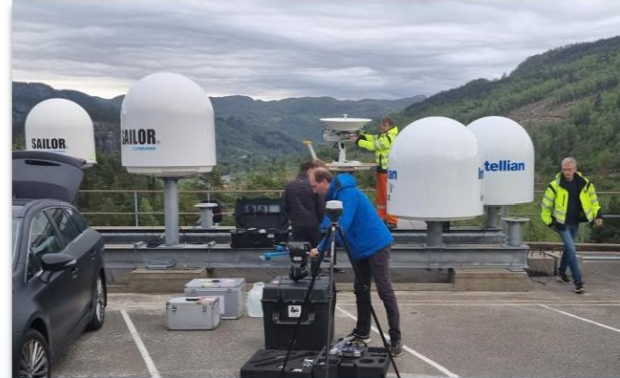
MARLINK – Norway, Eik Teleport Uts from 60cm to 1m – Ku band. Comparing gain between similar products.
